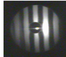
1/4 Wave Undercorrected Mirror With 1/2 Wave Turned Down Edge
